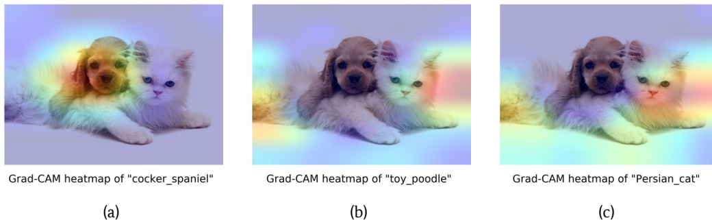
Figure 3: spaniel-kitty-paws-cut : Grad-CAM explanation of Inception V3 for the identification of the “cocker spaniel” (a), the “toy poodle” (b) and the “Persian cat” (c), when the paws are removed from the image (compare results of Fig. 2).
